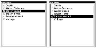
Options List for customizing Digital Data windows. The list appears with Water Speed selected (left). Temperature 2 has been chosen to replace Water Speed in the top digital data window (right).
